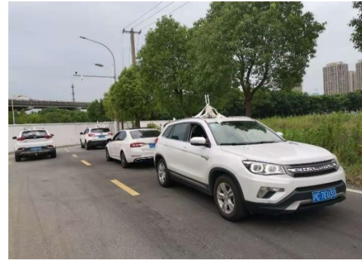
The OBU is placed on the top of the test car. The height of the antenna is about 1.5 m.
