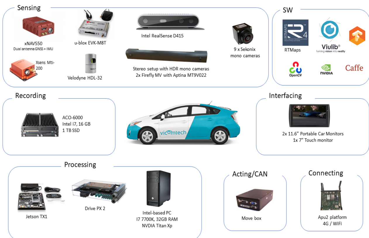
Figure 25: Overview of the HW and SW architecture of VICOM test vehicle
