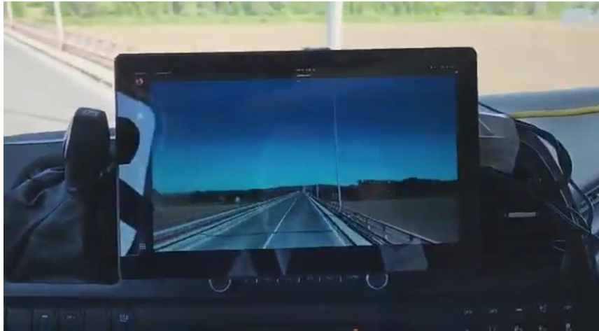
Figure 15: The SWIS screen on the follower truck presents the leader driver's view
