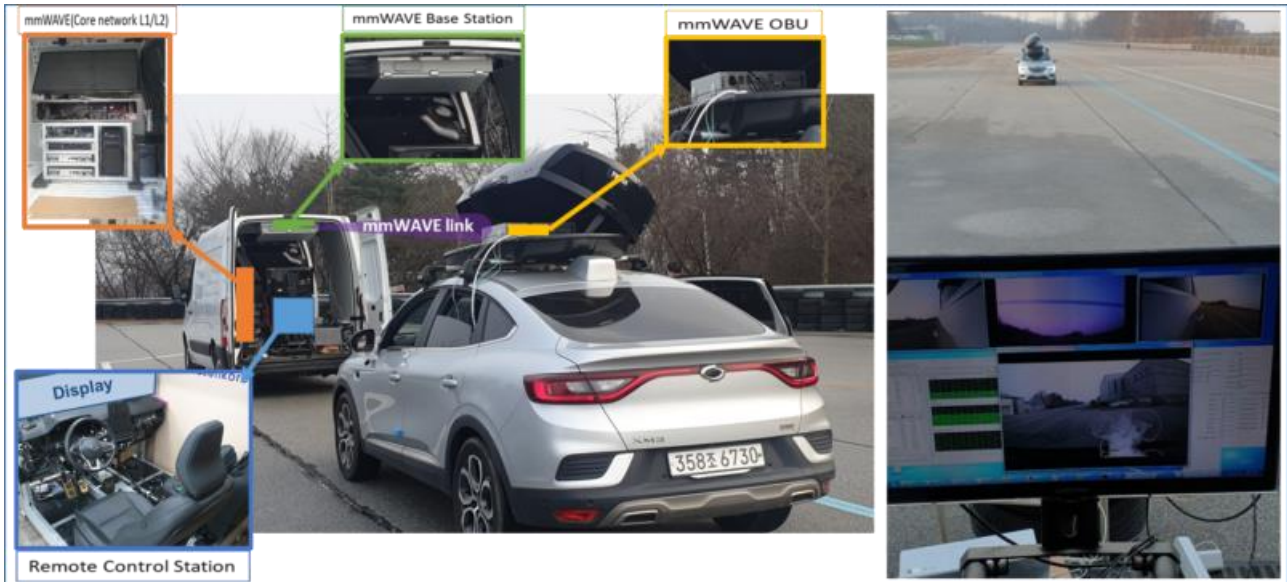
Figure 3: Field trial of the remote controlled via mmWAVE communication
