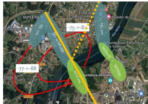
Figure 3 - 5G network handover configurations in ES-PT CBC
