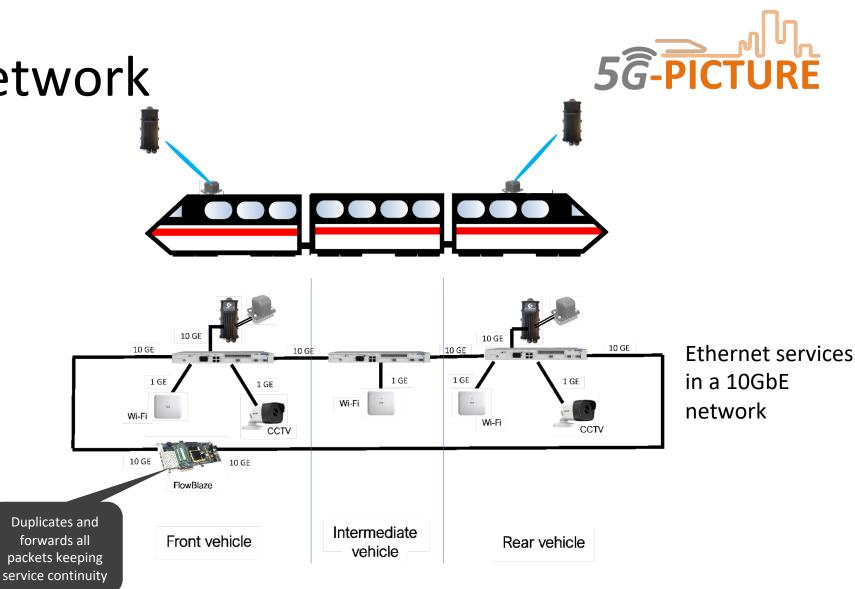
5G-PICTURE trial components on the Train Prepared for any FRMCS service support and coexistence with 5GNR
