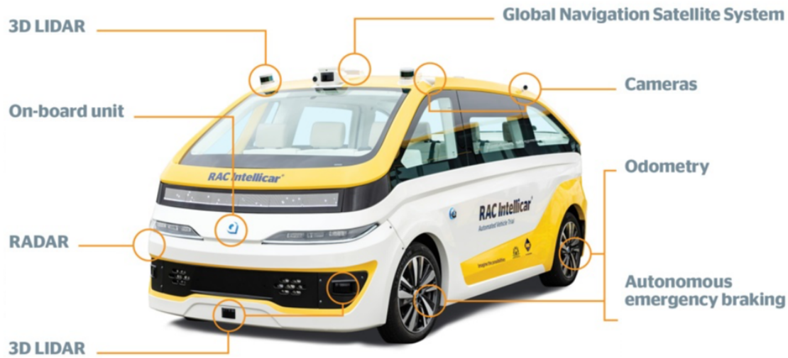
Figure 7: Sensors, cameras, and safety mechanisms of RAC Intellicar [32]
