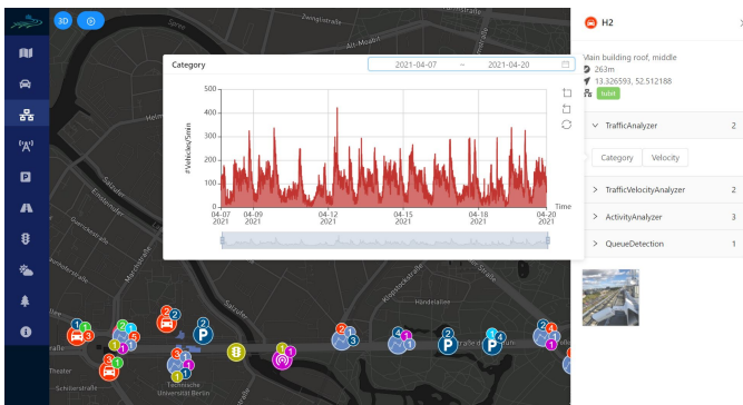
Fig. 1. Traffic pattern of legacy traffic detected by 5G-MOBIX roadside infrastructure at the Berlin trial site, shown within the control center application
