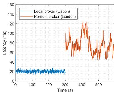
Fig. 9. MQTT broker location effect on latency for a stationary vehicle with QoS 0 and OBU to OBU scenario
