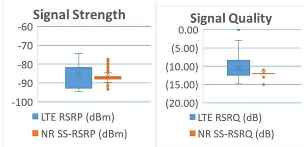
Fig. 4. Signal strength and Signal quality measurement
