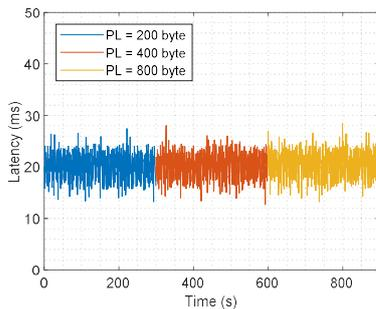
Fig. 8. Payload size effect on latency for a stationary vehicle with QoS 0 and OBU to OBU scenario
