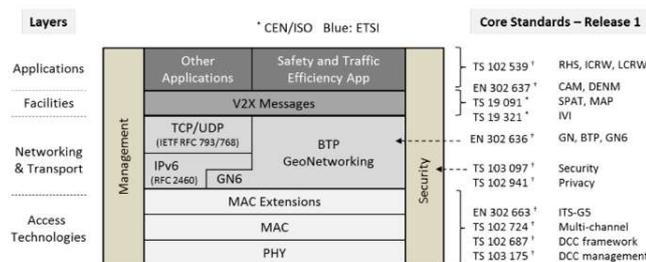
Fig. 1. C-ITS protocol stack (extracted from [1])
