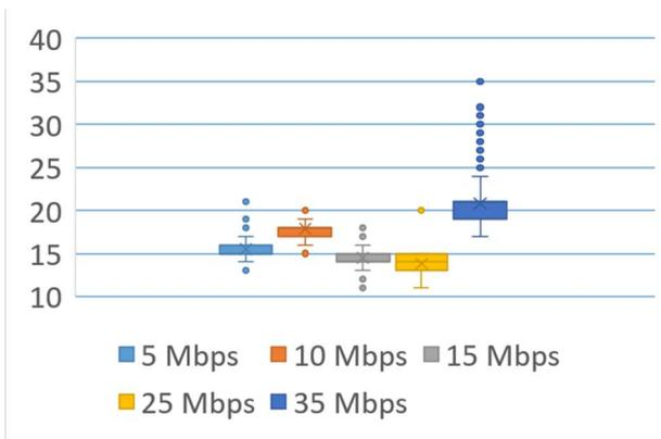
Fig. 5. One-way-delay OWD (ms) results (UDP DL)
