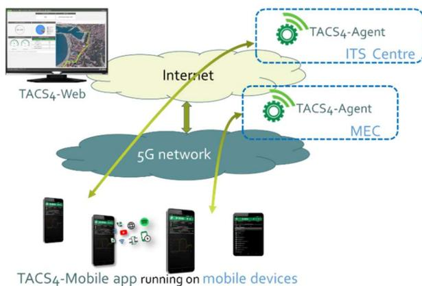
Fig. 2. Generic TACS4 Performance test solution overview
