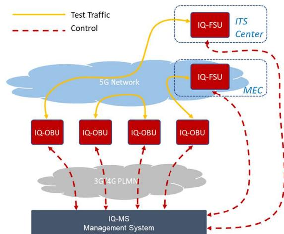
Fig. 3. IQ-NPE system architecture
