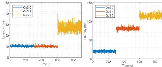
Fig. 7. a) QoS effect on message latency for a stationary vehicle (FSU to OBU), on the left; b) QoS effect on message latency for a stationary vehicle (OBU to OBU), on the right
