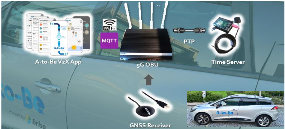
Figure 5 - Portuguese 5G Connected Vehicle architecture.
